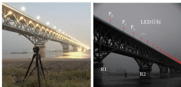
图 25 LED 辅助视觉测量 [35] Fig.25 Illuminated LED device aids visual measurement [35]
