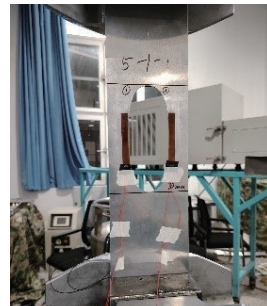
图13 壁板大开口试验件 Fig.13 Large-cutout panel test specimen
