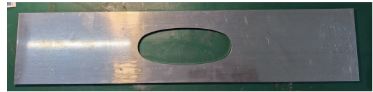
图13 壁板大开口试验件 Fig.13 Large-cutout panel test specimen
