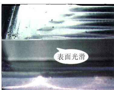
图 11 加工工艺优化后的加工工件表面 Fig.11 Surface of workpiece machined after process optimization
