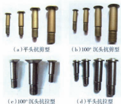
图4 北京航空制造工程研究所研制的英制轻型钛合金高锁螺栓 Fig.4 British system light-weight Ti-alloy bolt developed by Beijing Aeronautical Manufacturing Technology Research Institute
