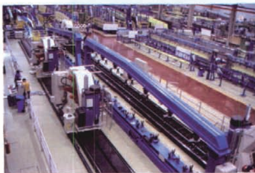
图3 并联机器人自动制孔 Fig.3 Automatic drilling of parallel robot
