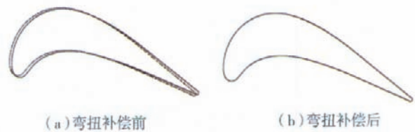
图8 弯扭变形的补偿 Fig.8 Compensation of twist deformation
