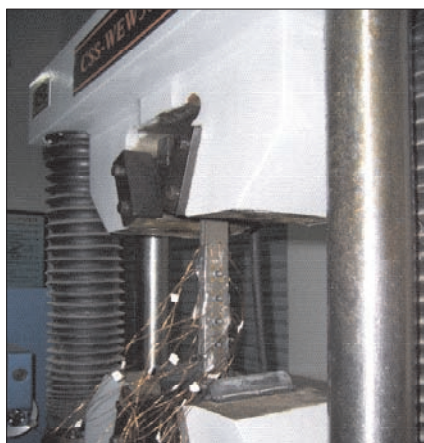
图5 钉载分配加载试验 Fig.5 Test of pin load distribution
