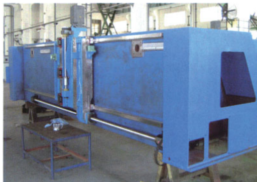
图2 轻型箱型梁(复材铺带机) Fig.2 Light-weight box beam (composite material tap-laying machine)
