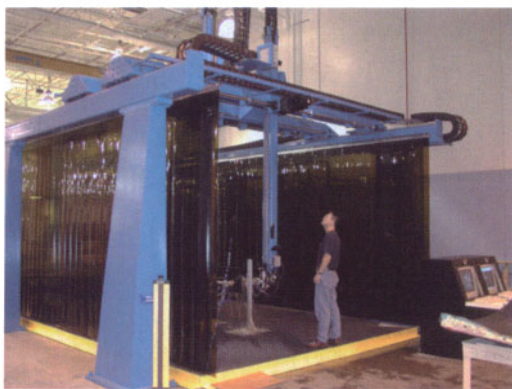
图4 穿透法C扫描三角型钢双纵梁 Fig.4 Through-transmission C-scan triangular steel double beam
