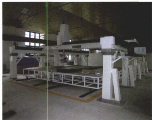
图1 CUS-6000大型超声自动扫描成像检测设备 Fig.1 CUS-6000 large-scale ultrasonic scanning imaging detect device
