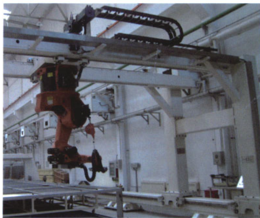
图3 矩形管等截面双梁(复材缝纫机) Fig.3 Rectangular tube constant dimension double beam (composite material sewing machine)
