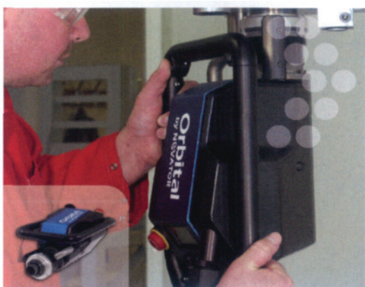
图2 Novator公司螺旋铣孔设备 Fig.2 Spiral milling equipment of Novator company
