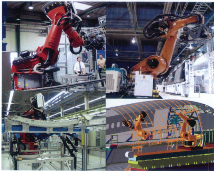
图6 基于工业机器人的自动制孔系统 Fig.6 Automatic drilling system based on industrial robot
