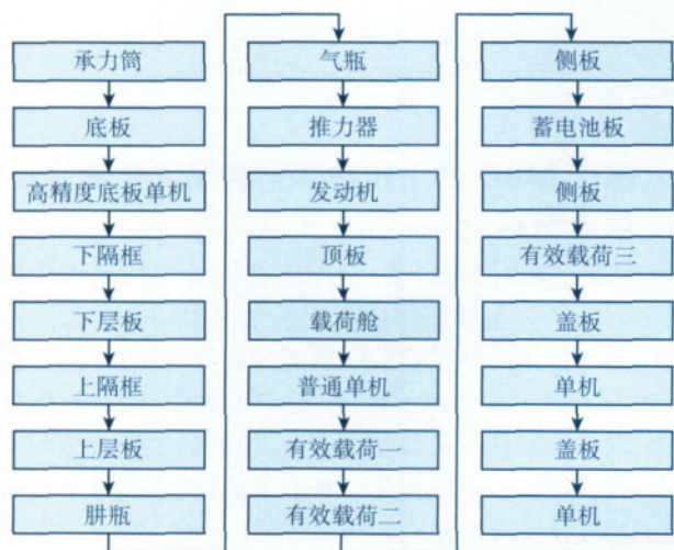
图8 某型号卫星装配顺序 Fig.8 Assembly sequence of a model satellite
