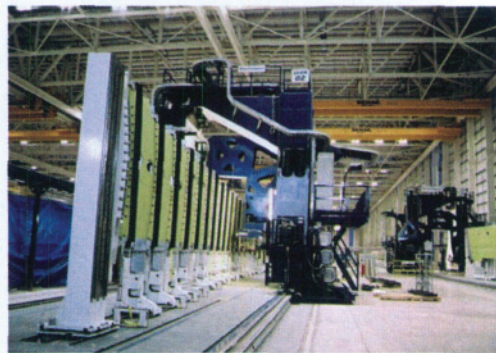
图2 以电磁铆接为动力的自动钻铆系统 Fig.2 Automatic riveting system based on electromagnetic riveting
