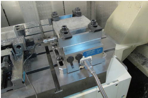
图8 振动传感器和测力仪的安装 Fig. 8 Installation of vibration sensor and dynamometer
