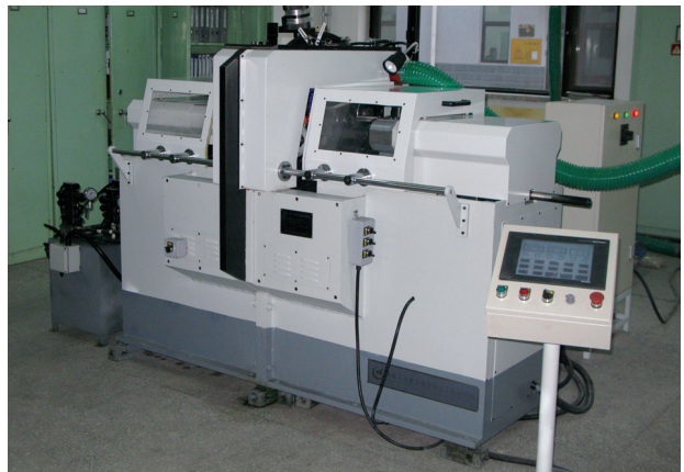
图5 SFP-300叶片双面抛光机床 Fig.5 SFP-300 blade double-sided polishing machine
