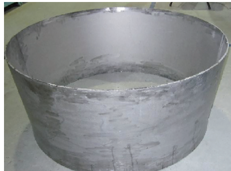
图2 气胀成形和热成型复合成形的筒体后段 Fig.2 Part by gas bulging and hot forming
