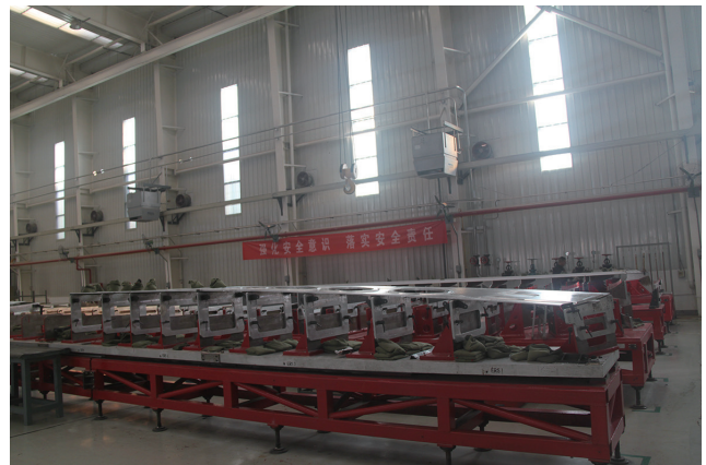
图1 厂房内机翼壁板喷丸检验夹具布局 Fig.1 Layout of the wing panels shot peening inspection fixture in the workshop
