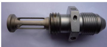
图5 钛合金管接头零件局部电镀镍 Fig.5 Parcel nickel-plating of titanium alloy pipe joint
