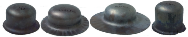
图4 500℃不同拉深深度钛合金零件 Fig.4 TA1 parts by hot granular medium forming process at 500℃
