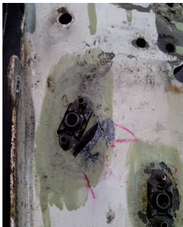
图4 货舱托板螺帽区域严重腐蚀 Fig.4 Severe corrosion around nut plate in cargo bay
