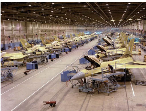
图2 F-16飞机固定机位式总装装配线 Fig.2 Fixed final assembly line of F-16
