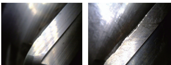
图11 山高刀具切削前后状态图 Fig.11 State of Seco before and after milling
