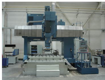
图1 SR240大型龙门多坐标仿形铣机床 Fig.1 SR240 multi-axis copying milling planer
