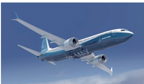
图8 B737MAX的双羽状翼梢小翼 Fig.8 Double feathery winglets on B737MAX
