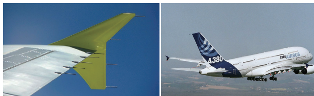
图6 A380的尖刀式翼稍小翼 Fig.6 Knife-winglets on A380
