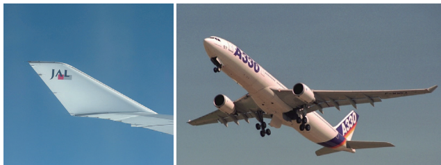
图4 A330的梯形翼稍小翼 Fig.4 Trapezoid winglets on A330
