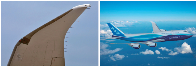
图7 B747-8I的斜削式翼梢小翼 Fig.7 Raked-winglets on B747-8I
