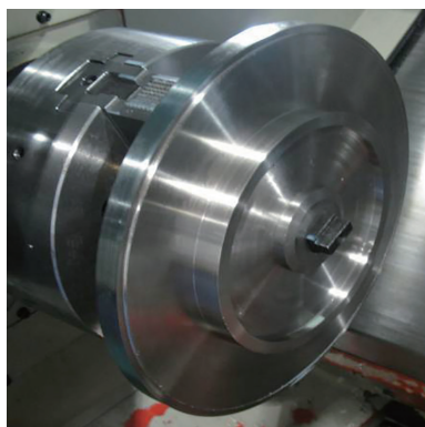
图3 GH4133B发动机涡轮盘 Fig.3 GH4133B engine turbine disc
