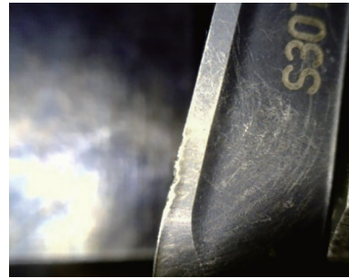
图6 Sandvik S30T磨损 Fig.6 Wear of Sandvik S30T
