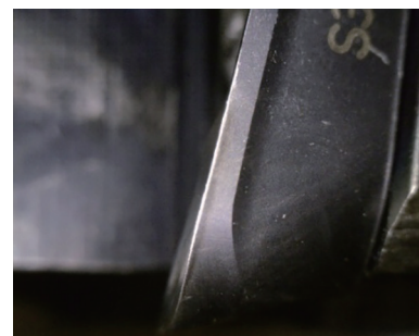
图7 Sandvik S30T后刀面钛化合物亲和现象 Fig.7 Titanium compound affinity of Sandvik S30T in flank face
