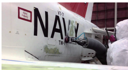
图7 采用移动式工业机器人进行飞机退漆 Fig.7 Aircraft exterior de-painting system with robot
