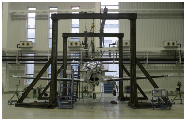
图7 复合材料飞机地面共振试验 Fig.7 Ground vibration test of composites aircraft
