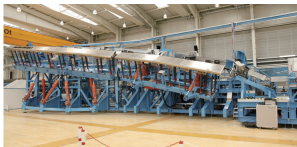
图3 A350飞机高升力系统集成试验台 Fig.3 Integration test rig for A350 high lift system
