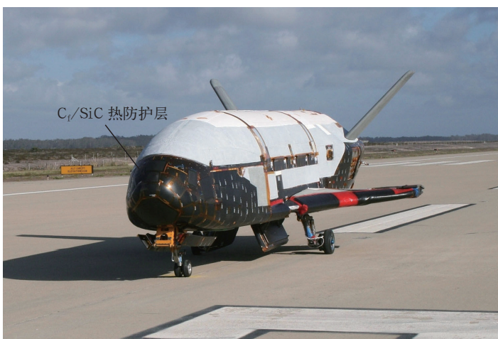
图1 X-37B航天飞行器上的C f /SiC热防护层 Fig.1 C f /SiC thermal protection layer in X-37B aerospace craft
