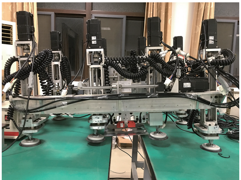
图3 爬行机器人制孔系统 Fig.3 Crawling robot drilling system
