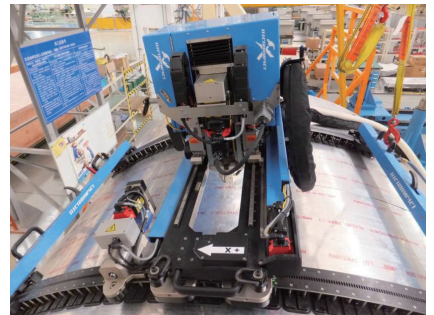
图2 柔性轨道制孔设备 Fig.2 Flexible track automatic drilling machine
