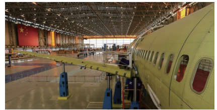
图5 机翼与机身调姿对接 Fig.5 Attitude adjustment and butt joint of wing and fuselage
