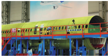
图4 前机身与中机身调姿对接 Fig.4 Attitude adjustment and butt joint of the forward fuselage and the main fuselage
