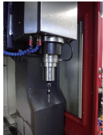
图16 大连理工大学研制的超声振动刀柄 Fig.16 Tool holders for ultrasonic assisted machining developed by Dalian University of Technology
