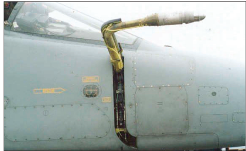
图13 狂风摇臂式受油装置(座舱右前方) Fig.13 Fuel receiving device by rocker of Tornado (right front of the cockpit)
