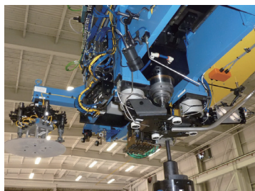
图6 GEMCOR 自动钻铆系统末端执行器 Fig.6 End-effector of GEMCOR automatic drilling and riveting system
