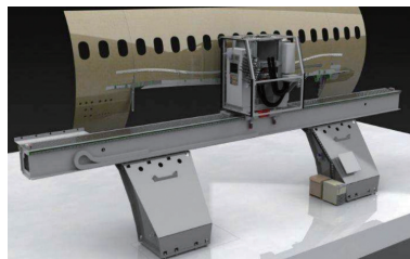
图3 自动钻铆一次装配系统 Fig.3 One time assembly system of automatic drilling and riveting
