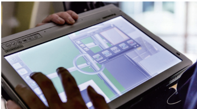
图4 MiRA正在用于检测可以固定液压系统、管路的结构支架 Fig.4 MiRA is being applied to check the structural brackets that hold systems such as hydraulics and pipes in place
