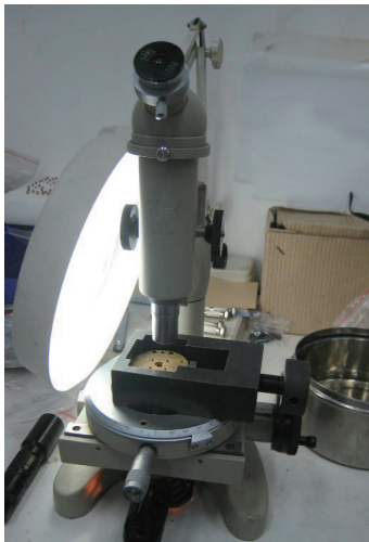
图3 显微镜下精压喷嘴 Fig.3 Push the nozzle under the microscope
