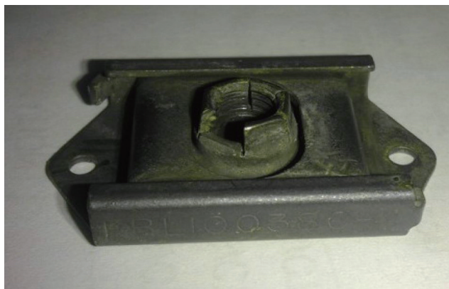
图6 损坏的托板螺帽 Fig.6 Damaged nut-plate
