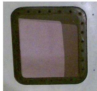
图5 口框密封剂就地硫化图 Fig.5 Vulcanization diagram of hatch sealant
