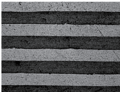
图4 Ti/Al层状复合材料SEM扫描图像 Fig.4 SEM scan image of Ti/Al laminated composites
