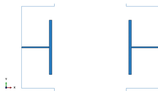
图5 钳头简化有限元模型 Fig.5 Simplified finite element model of jaws
