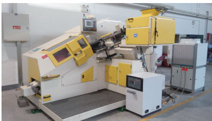
图4 数控温搓丝机 Fig.4 Numerical control warm rolling machine
