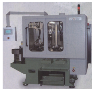
图5 自动数控攻丝机 Fig.5 Automated numerical control thread tapping machine
