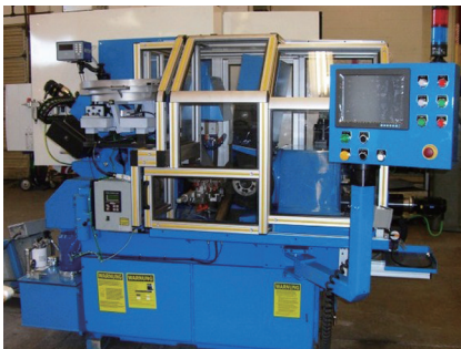
图3 自动上料的数控无心磨床 Fig.3 Numerical control centerless grinder machine with automated loading
