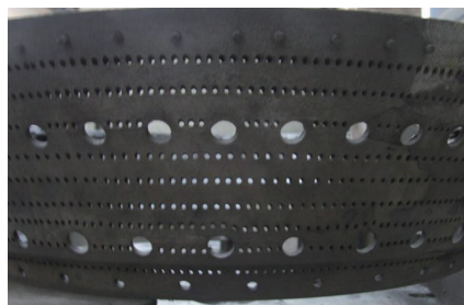
图1 传统机械加工的CMC-SiC复合材料构件 Fig.1 CMC-SiC composite structure machined by traditional technology
