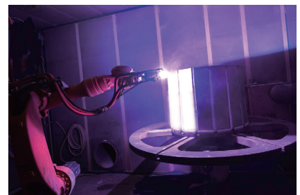
图1 机器人自动喷涂发动机部件热障涂层 Fig.1 A robot-operated plasma spray TBCs for engine components
