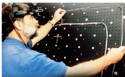
图2 波音公司开发的AR布线试验系统 Fig.2 AR wiring test system developed by Boeing company
