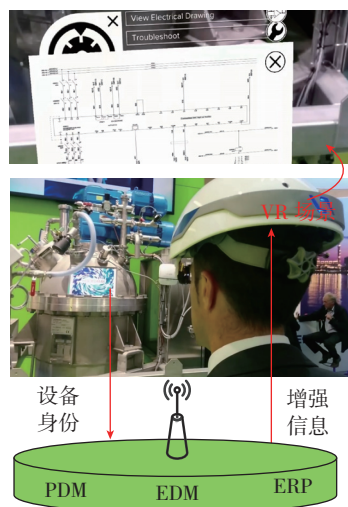
图11 基于AR的全息索引 Fig.11 Entire manufacturing information index based on AR
