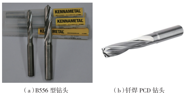
图1 肯纳金属有限公司的B556型钻头和钎焊PCD钻头 Fig.1 B556 and brazing PCD drilling tools of Kenna Metal Co., LTD
