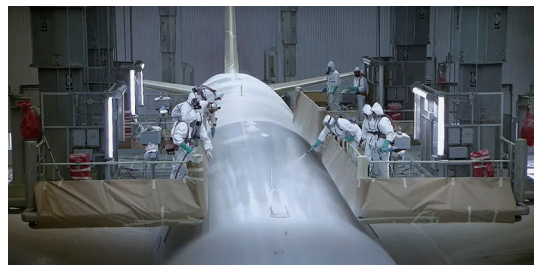
图1 波音公司的辅助喷涂系统 Fig.1 Assistant painting systems of Boeing SAFARI
