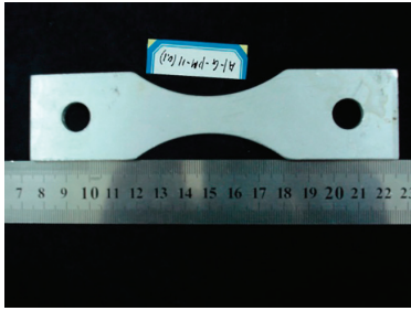
图7 抗疲劳裂纹萌生 (S-N曲线) 试样 Fig.7 Specimen dimension of S-N test
