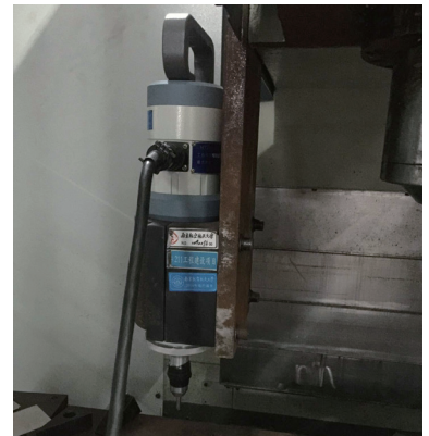
图3 超声波数控成形与校形装置 Fig.3 Ultrasonic CNC forming and straightening device
