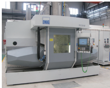
图1 EMAG六轴精密振动电解加工设备 Fig.1 EMAG PECM machine with six axes
