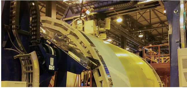
图1 E7000自动钻铆系统 Fig.1 E7000 automatic drilling riveting system
