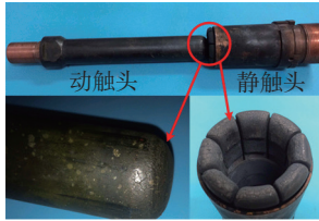
图9 CuW电触头表面龟裂失效形貌 Fig.9 Surface crack morphology of CuW electrical contacts
